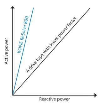
If the power factor is poor - if there is a lot of reactive power and less active power - there will be more heat loss and larger fuses will be required. With its high power factor, the KONE ReSolve 800 minimizes heat loss and increases the lifetime of the equipment.
